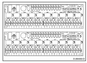
Figure 6-34 Twenty-Relay Dry Contact Kits
